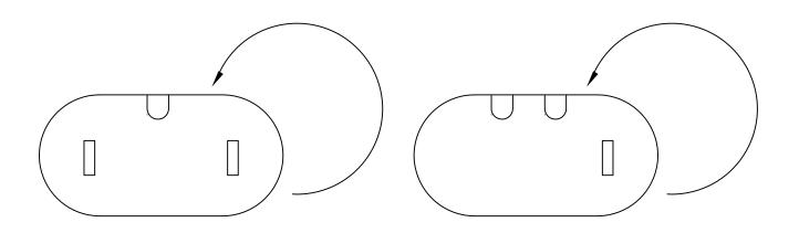
THE SOFT RUBBER PLUG ON THE HEADLIGHT ADAPTER HARNESS WILL ALLOW IT TO BE INSERTED INTO THE OEM HARNESS "UPSIDE DOWN."
